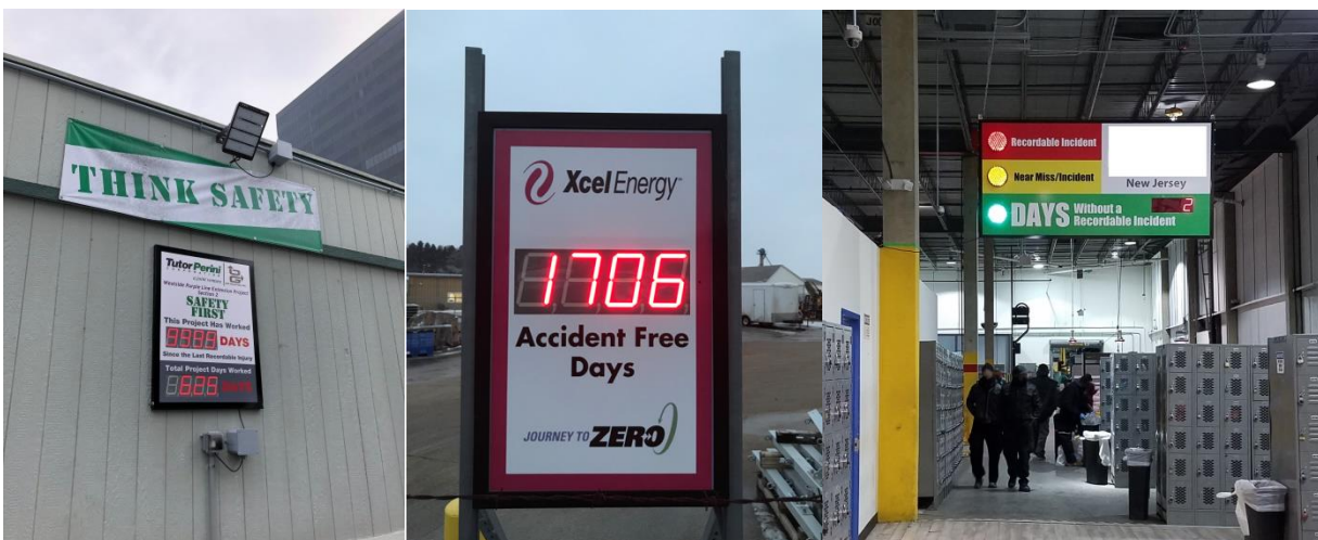
Examples: Left to right: bracket or bolt through backer, post mount through enclosure side, hanging mount
